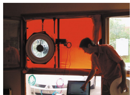
Measure of the air permeability of a building with the principle of the blower door
